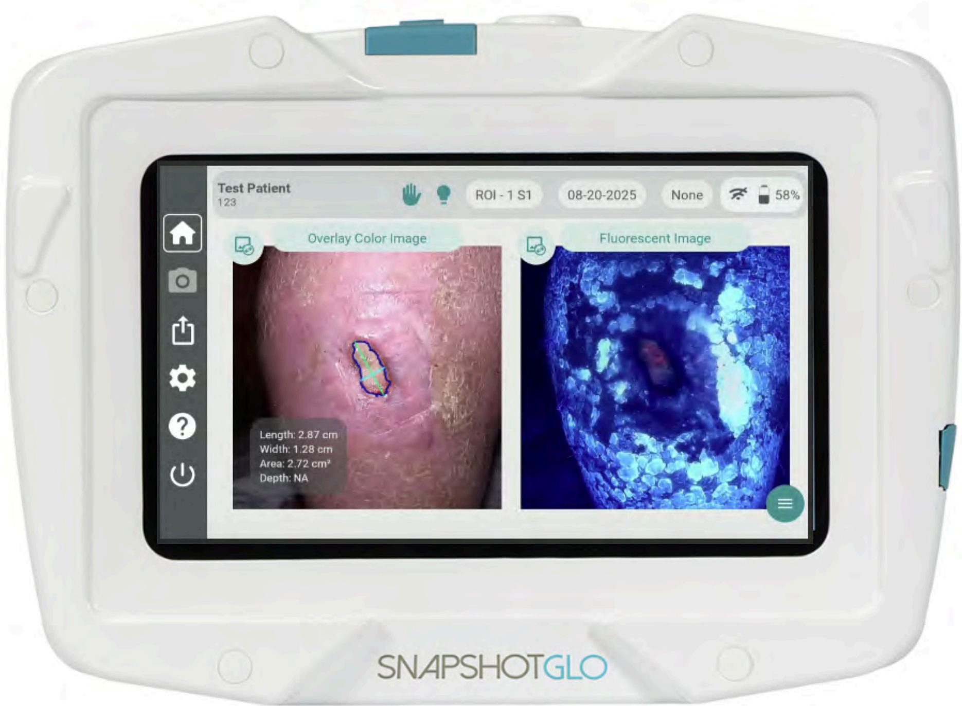
Figure 1: SnapshotGLO device displaying RGB image (L) with wound measurement alongside BAF image (R) side by side.
